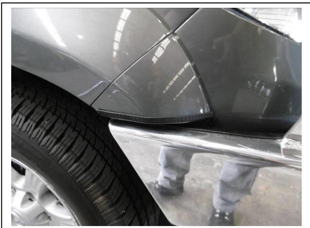
Figure 11: Flare, cut and installed
