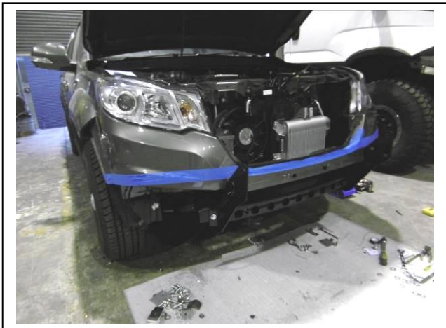
Figure 9: Cut line on bumper. Lower side of tape line
